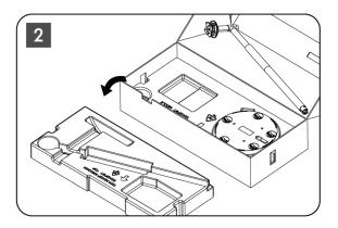
3. From the second layer, take out the TV mount base, which has built-in wheels, and place it on its side.
