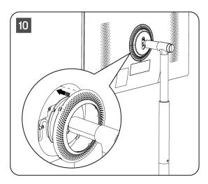
**Note:** Make sure that the mains cable is properly plugged into the TV set and does not prevent the cover ring from closing.
