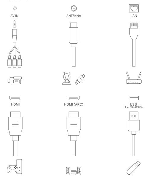
Open the port dust cover and connect to the corresponding port as per need:
